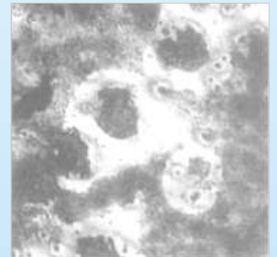
SG Core Photomicrograph X100 (Hs 35-45 °ShC)
